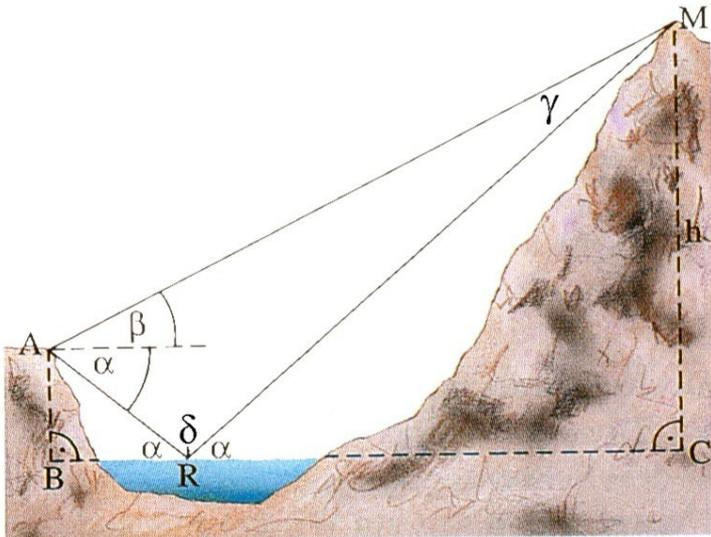
$$\overline{AR} = \frac{h_{\text{See}}}{\cos(90^\circ - \alpha)} = \frac{120\text{m}}{\cos(78,2^\circ)} = 586,81\text{m}$$
